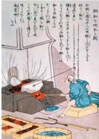
"Nanban-buki," an ancient smelting technique that used lead to separate silver and remove impurities contained in black copper. The technique is described in detail in the Kodo Zuroku (Illustrated Book on the Smelting of Copper) issued by the House of Sumitomo at the beginning of the 19th century.
