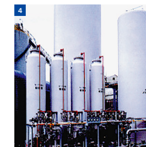
3. Packaged methanol reforming high-purity hydrogen gas generator (100Nm 3 /h, 99.999% purity), used by customers requiring high-purity hydrogen, such as in semiconductor manufacturing. 4. H 2 -PSA hydrogen gas purification system. Hydrogen gas is recovered by decomposing methanol or natural gases.
