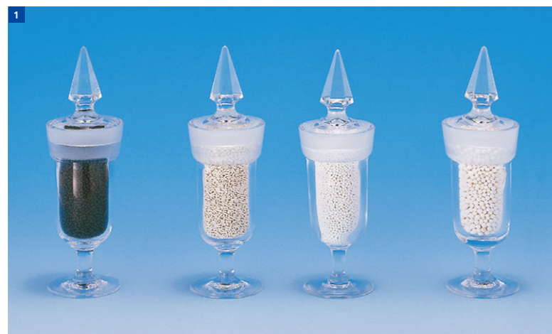
1. In PSA, various adsorbents, including synthetic zeolites, are used depending on the target gas. 2. Sumitomo Seika Chemicals, which began as a manufacturer of fertilizers and functional chemicals, has since distinguished itself in the gas business. Its strength lies in its ability to tailor systems to customer needs, from compact units to large-scale installations.
