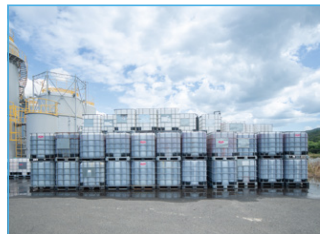
Ume seasoning effluent in 1m³ containers. Nakata Foods alone produces 10m³ of effluent per day.
