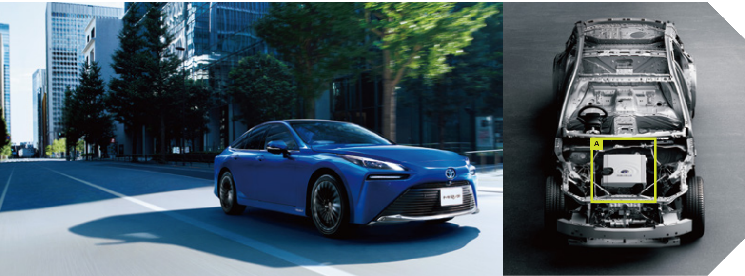
The new Mirai, Toyota Motor’s latest FCEV featuring Sumitomo Riko seal components. A box (A) in the photo above indicates the fuel cell stack where electricity is generated.
