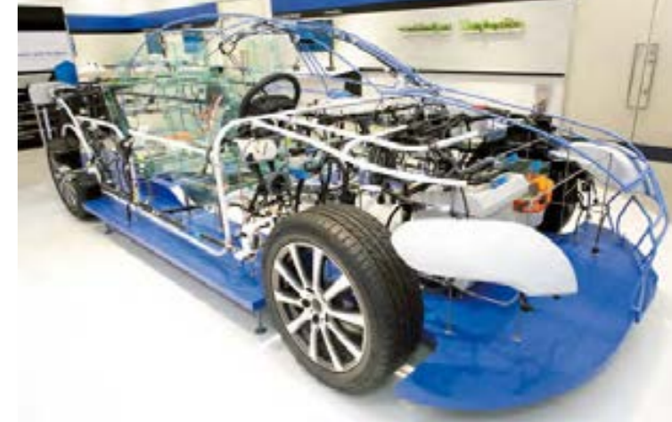
This skeleton of a car displayed in the showroom at Yokkaichi Plant shows that wiring harnesses are everywhere. As automobiles evolve, they incorporate more and more novel components. The guts of a car are becoming increasingly complex.
