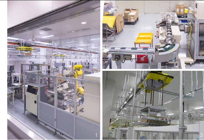
(1) A team of robots packaging drugs. (2) Packs of the most widely prescribed diabetes drug in Japan travel along a conveyor. (3) A robot nicknamed Sky Love carries packaged drugs overhead.
