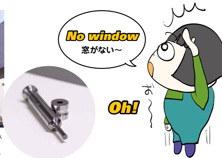
A windowless building where solid formulations are produced (above). A punch and a die from a tablet press (right). 窓のない新固形製剤棟の外観(上)。打錠機に組み込んでいる、きねと臼(右)。
