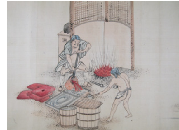
Producing teido copper plates at the Tatsukawa Refinery early in the Meiji era (Part of a scroll painting depicting the Besshi Copper Mines from the collection of Sumitomo Metal Mining).
